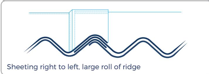
If the 2 piece close fitting ridges is sited the opposing way then the lap of the ridge must be offset 1 corrugation from the lap of the sheets.
